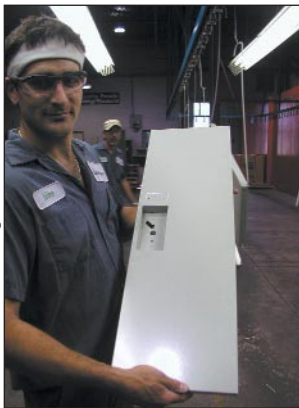
A Hadrian employee does a quality inspection on a locker.
