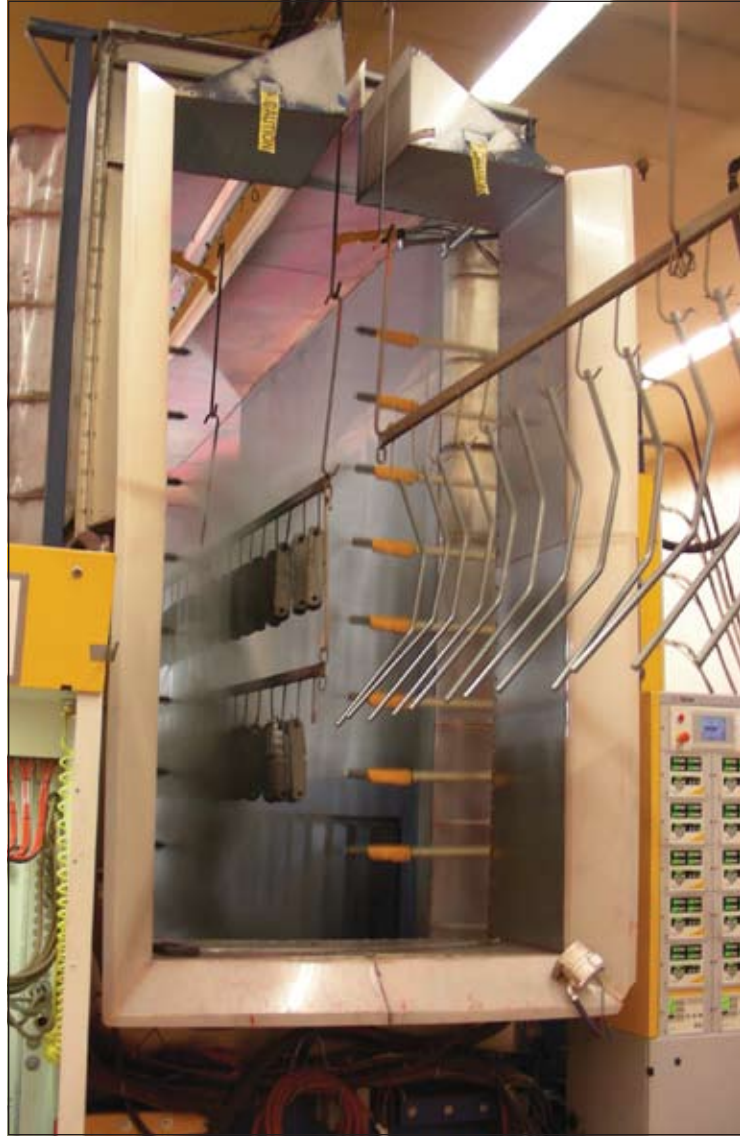
Colour change time has been reduced on the continuous flow powder line at agricultural equipment maker Case New Holland.
