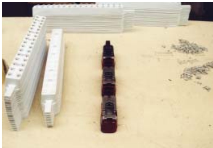
Molded part holders are inexpensive and hold parts securely during the coating and curing operations.
