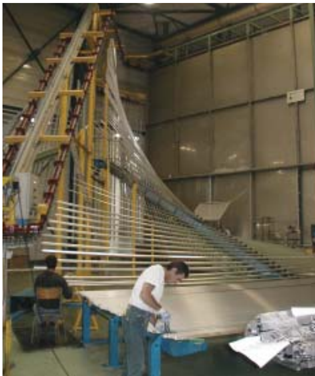
An automated loading system provides simple loading with limited labor at SFPI's custom coating shop in Fougères, France.
