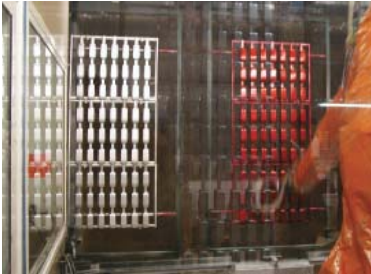
A robot applies all of the liquid coatings.
