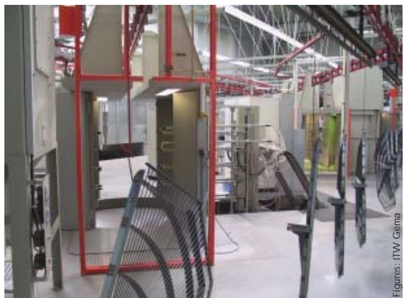
At Wanzl, the two automatic booths and one manual booth were arranged at an angle to each other. The chain speed is 4 metres per minute.
