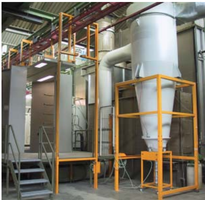
Height-adjustable pedestals for manual coating at Karl Miller avoid fatigue during precoating and touch-up coating.
