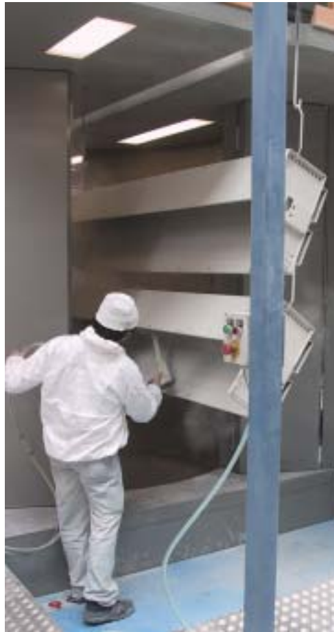
At Megamat, one quick-change booth is used in the classic manner for colour changes and a second is used mainly as a single colour system.
