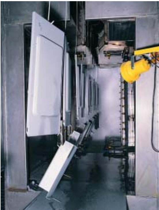
The seven-stage pretreatment system has helped improve corrosion resistance on parts.
