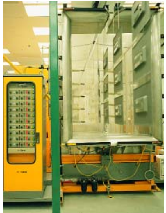
The spray booths, controlled by Compact PLCs and Graphic Magelis operator interfaces, have a mini cyclone system capable of multiple colour recovery with virgin color feed.
