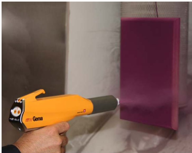
Powder Coating of MDF Cabinet Door
