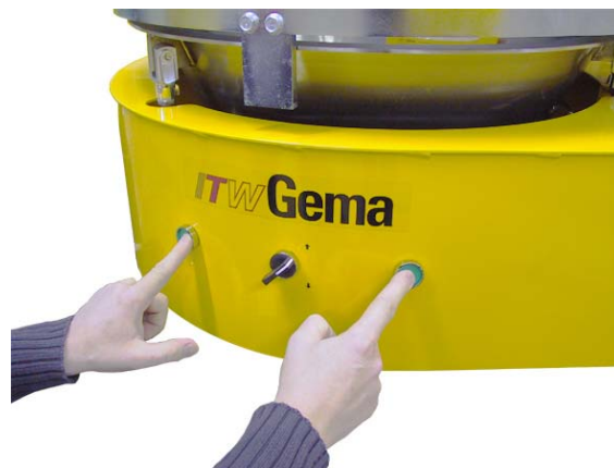
Two-hand security-operation of the delivery unit
