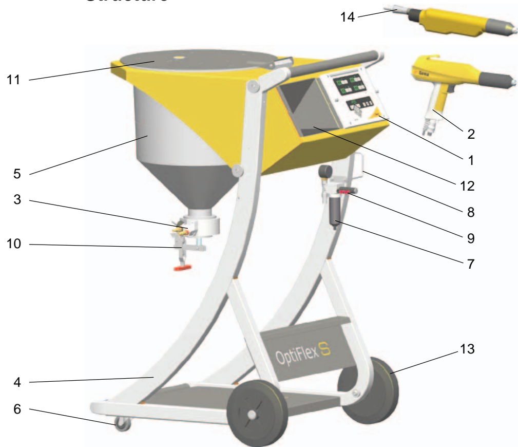
OptiFlex BN Powder coating equipment - structure
